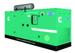
The acoustic enclosure is made of 1.6 mm thick CRCA sheets in Munsel green shade and a structural/ sheet metal base frame painted in black. The walls of the enclosure are insulated with fire retardant foam so as to comply with the 75 dBA at 1 mtr sound levels specified by Ministry of Environment & Forest.
